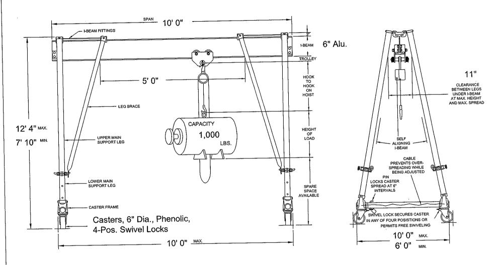
Aluminum Round Tube Frames and Aluminum I-Beam
