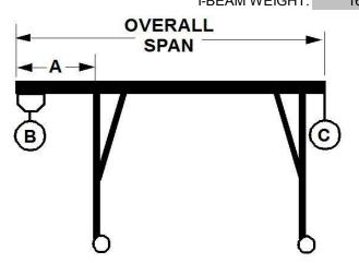
PROPER CANTILEVER PROCEDURES Required counterweight should not be supported by gantry caster frame.
