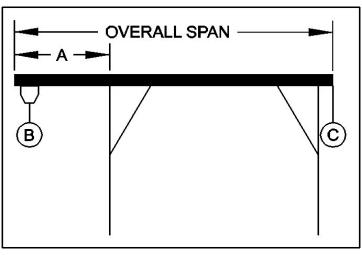
PROPER CANTILEVER PROCEDURES Required counterweight should not be supported by gantry caster frame.
