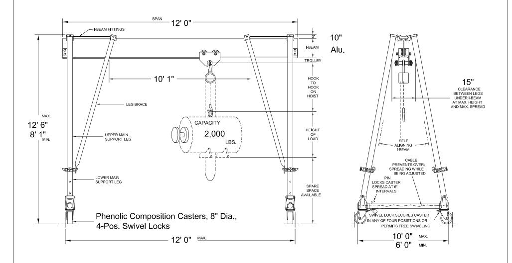
Round Tube Aluminum Frames and Aluminum I-Beam
