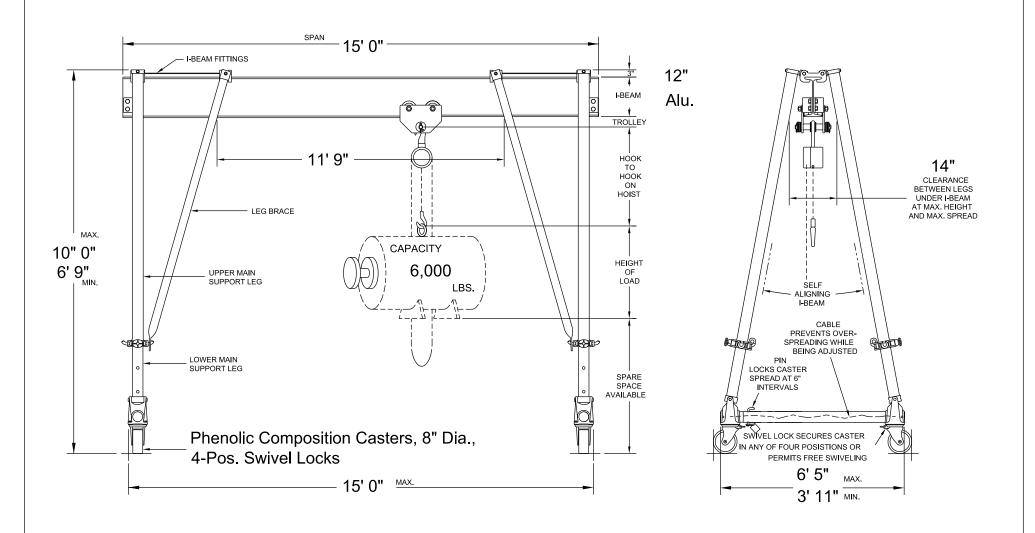
Round Tube Aluminum Frames and Aluminum I-Beam
