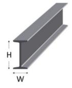
I-Beams (named because of their shape) provide great load-bearing support.
