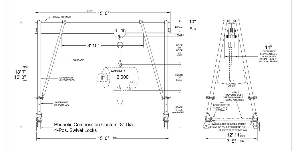
Round Tube Steel Frames and Aluminum I-Beam
