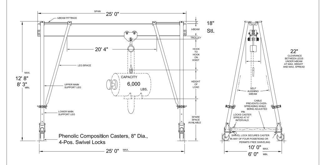
Round Tube Steel Frames and Steel I-Beam
