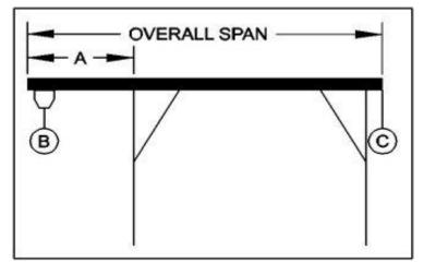
PROPER CANTILEVER PROCEDURES Required counterweight should not be supported by gantry caster frame.
