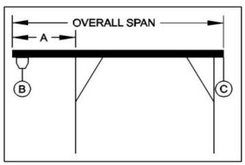
PROPER CANTILEVER PROCEDURES Required counterweight should not be supported by gantry caster frame.
