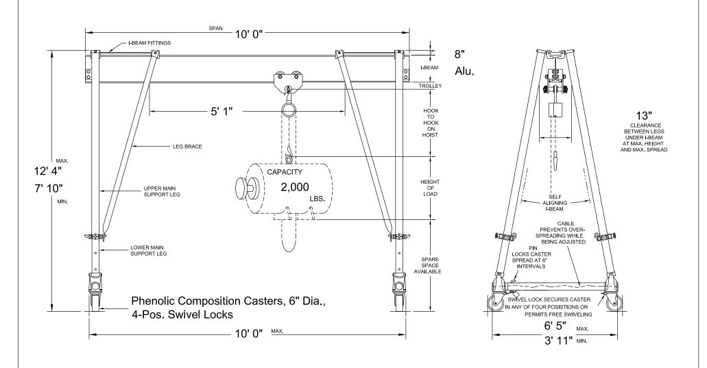
Round Tube Steel Frames and Aluminum I-Beam
